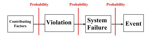
Figure 4. Event Model 1 with a Violation Leading Directly to a System Failure
